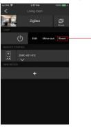
From your ZigBee controller or hub interface, choose to delete or reset the lighting device as instructed. The connected light blinks 3 times to indicate successful reset.
